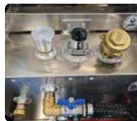
2 "analog level gauge, 2" tank cap, 1 "pressure / vacuum release valve.
