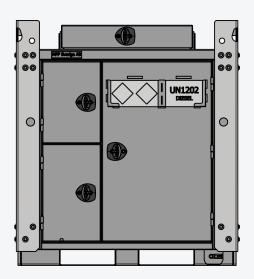
The cabinet doors are equipped with rubber seals to prevent dust and dirt from entering and have built-in locks that can be padlocked.
